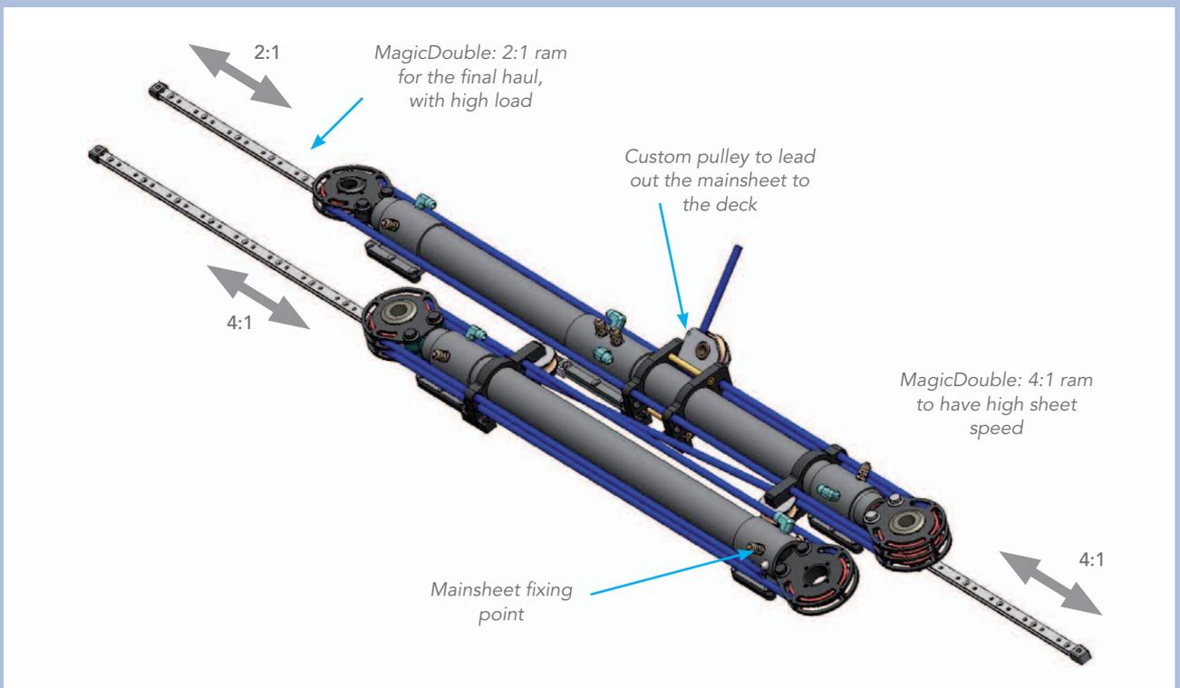
The mainsheet Magic Trim + Magic Double system developed for a Swan '60. Trim sequence: both cylinders closed, Magic Trim start to exit, than starts the 4:1 side of Magic Double tacking the mainsheet speed. When the 4:1 side of Magic Double is fully extended and the load of sheet increases, the 2:1 Magic Double ram completes the hauling of the sheet. Vice versa for easing sequence.
