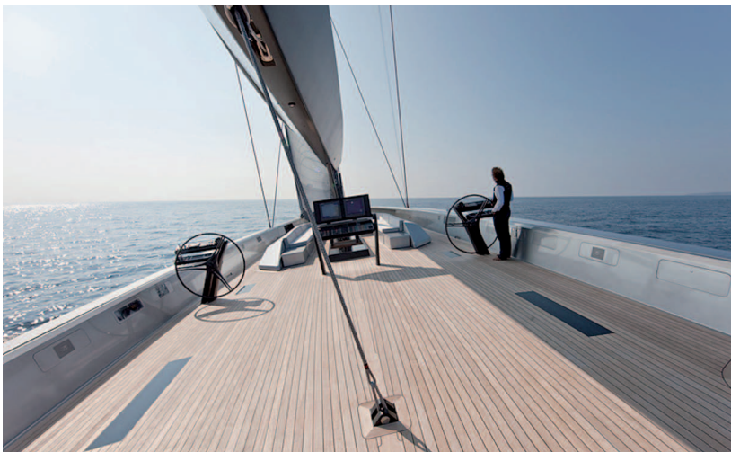
Wally 130' deck: Smart MagicTrim and MagicDouble are used for mainsheet and jib sheet. Thanks to these automatic systems, the deck is flush and free from winches and their sheets.
