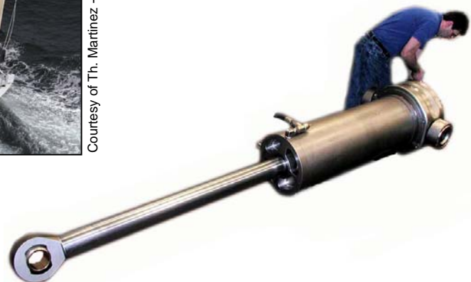
MARI-CHA IV canting keel cylinder onboard with the special asymmetrical bearing.
