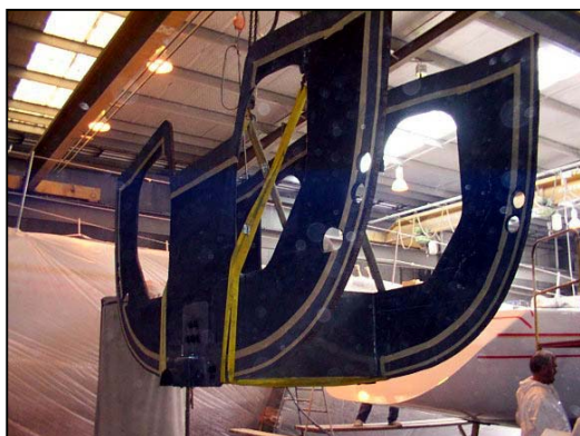
Bulkheads with keel jig during assembling with the hull
