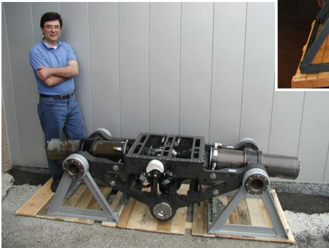
60' canting keel system 160 mm bore. Cylinder tube and components made of black hard coated aluminium (Ergal 7075), piston rod and terminal in 17-4-PH H900 SS. Bearings in Ergal 7075 and 17-4-PH H900.
